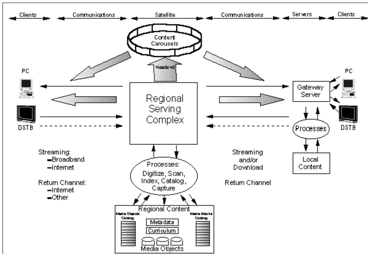
**Figure 1.** Diagram of the EduPort end-to-end integrated solution architecture.
