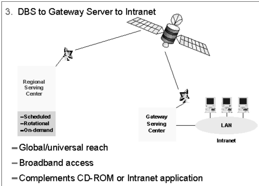
**Figure 3.** PC or other Gateway/Server connected to DBS and an intranet
