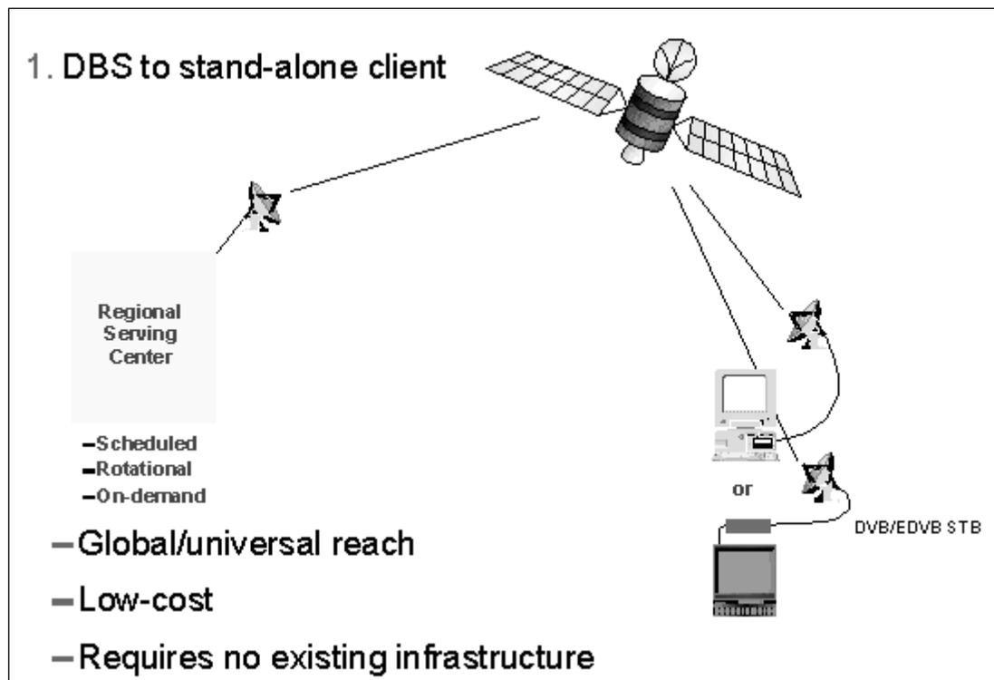
**Figure 1.** Single stand-alone PC or TV client with access only to DBS.
