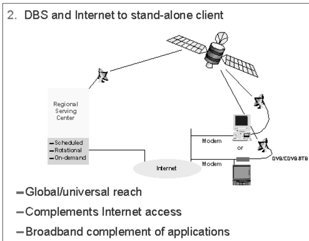
**Figure 2.** Single PC or TV client with access to both DBS and the Internet.
