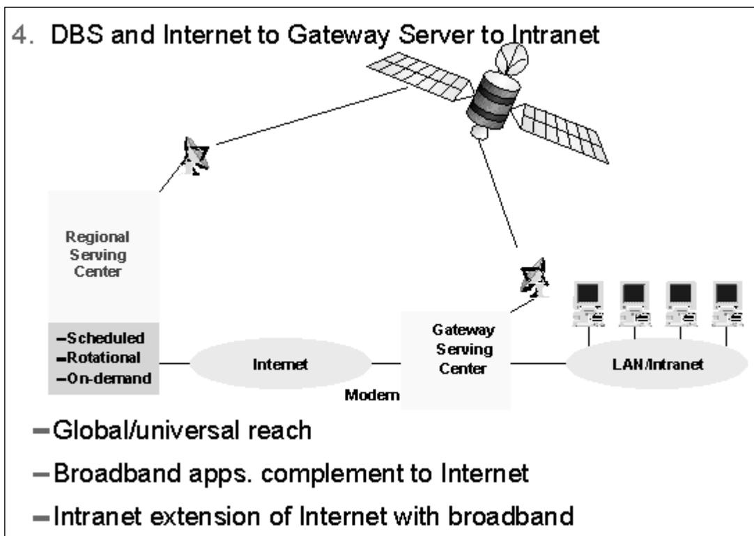
**Figure 4.** PC or other Gateway/Server connected to both DBS and the Internet and an intranet
